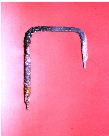
**Figure 5.** Corroded rebar from a 4 years old building in hot and salty environment
