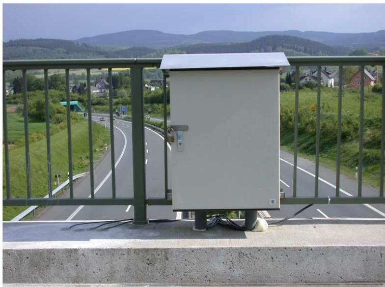
**Figure 14.** Measuring unit of exposure tests at a highway in Germany within the splashwater zone
