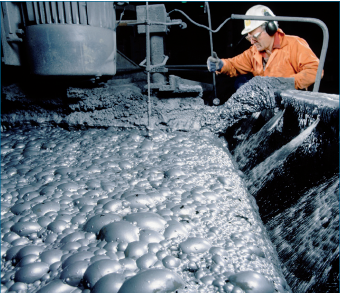
Fig. 9: flotation cell in mineral processing (Clariant)
