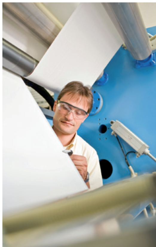
Ceramics by the yard: ceramic separators enhance the safety of lithium-ion batteries (© Evonik)
