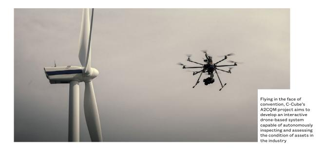
C-Cube, in collaboration with HighlightDynamics and Helvetis, are initiating a project named A2CQM, which aims to develop an interactive drone-based system capable of autonomously inspecting and assessing the condition of assets in the industry.
