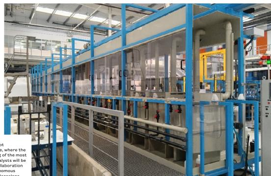
CIDETEC's pilot production line, where the manufacturing of the most promising catalysts will be upscaled in collaboration with the Autonomous University of Barcelona
