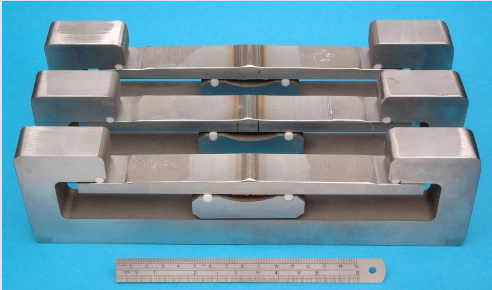
Specimen 210L x 25W x 10T mm
