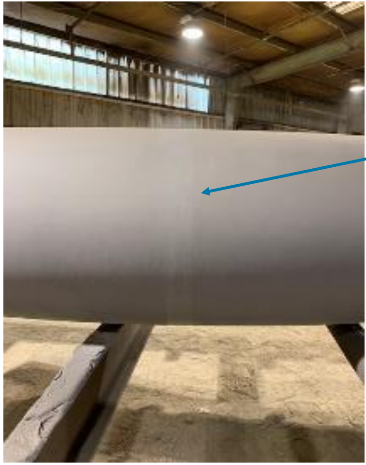
PPG HI-TEMP 1027 HD gray, 24 hours after application
