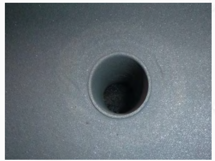
Nozzle after surface preparation
