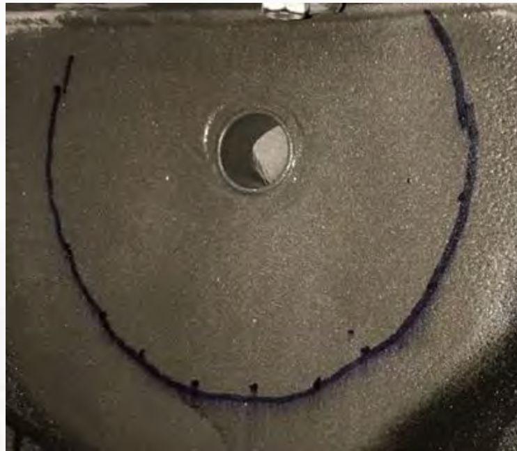
Nozzle after HVTS application
