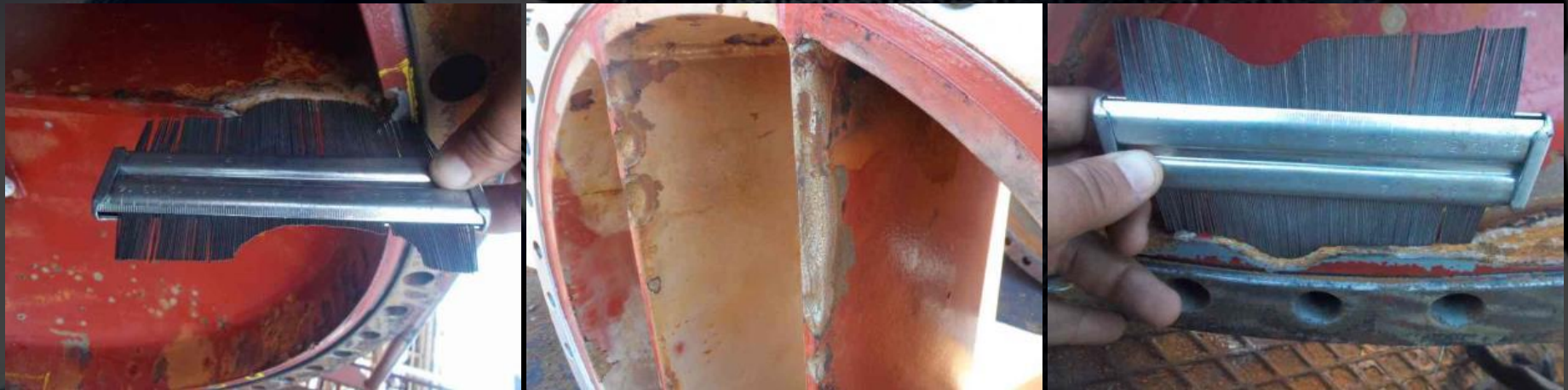
Interaction between bundle in titanium and chambers in carbon steel
