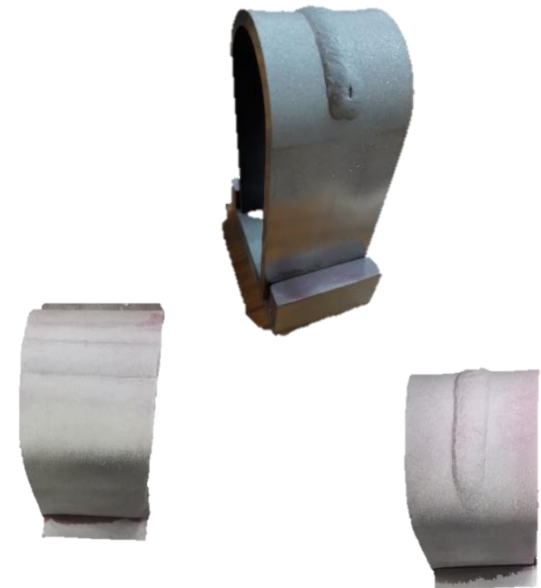
Weld in transverse direction
