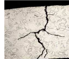
Stress Corrosion Cracking (austenite) High temperature
