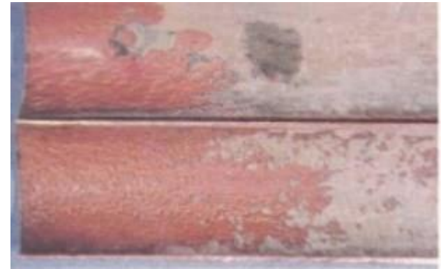
Tube inlet erosion-corrosion http://heatexchan.blogspot.com/2017/12/heat-exchangers-chemically-induced.html?_sm_au_=iPVQDQjWNrsPJJJs
