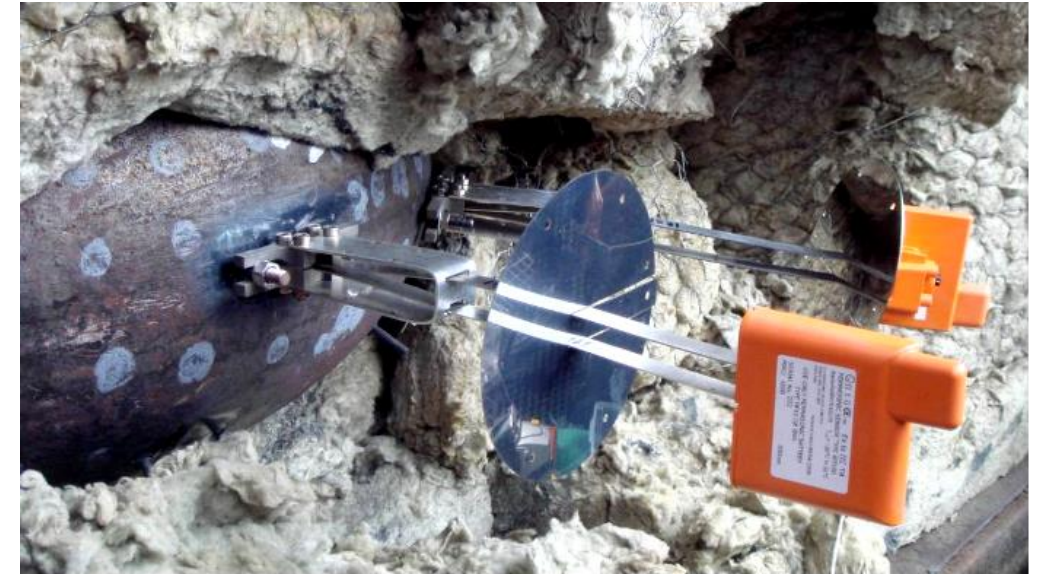
Figure 1: Probes installed on cast carbon steel U-bend with M8 studs
