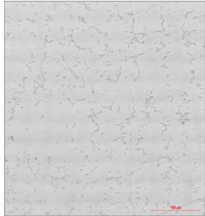
RECORD EST 625-1 LD cladding as welded. From left to right: fusion line area, middle of the bead. Austenitic matrix with some Mo precipitates typical for Alloy 625 - Electrolytic etching 10% \text{Cr}_2\text{O}_3
