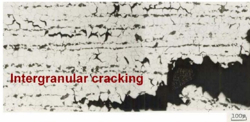
Cross section of HTHA elbow
