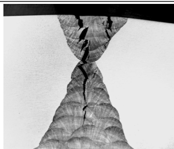
Severe cracking in weld metal
