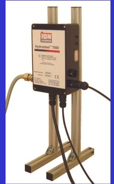
Continuous Active Corrosion and HIC risk Measurement Mapping hydrogen flux over time in high criticality areas
