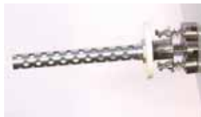
HT-R High temperature (<500 °C) roaming probe.
