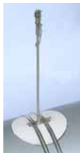
AT-S stationary probe for routine spot measurements and continuous monitoring
