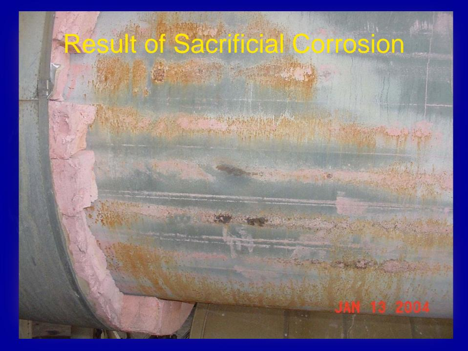
Novalac Epoxy After 3 months service Originally White Cracking Excessive DFT in places.
