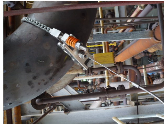
HT350 Transducer installed on an Elbow before Insulation re-instatement
