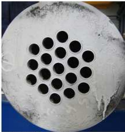
Tubesheet after rolling
