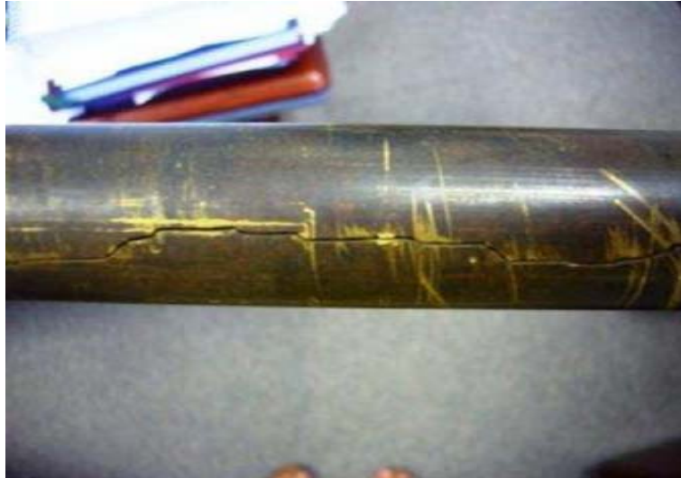
Tube cracking at middle area by ammonia SCC
