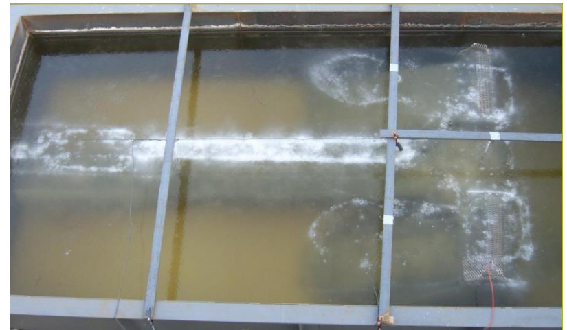
Anchor in polarized alkaline bath, A-Corros®
