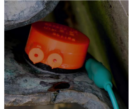
Electrochemical measurements on bronze artefacts - POLITO®
