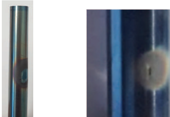
Figure 3 - Pinhole cracks on the surface of Zircaloy-4 cladding tubes caused by ISCC [2]
