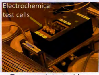
Thermostatic bath with electrochemical test cells
